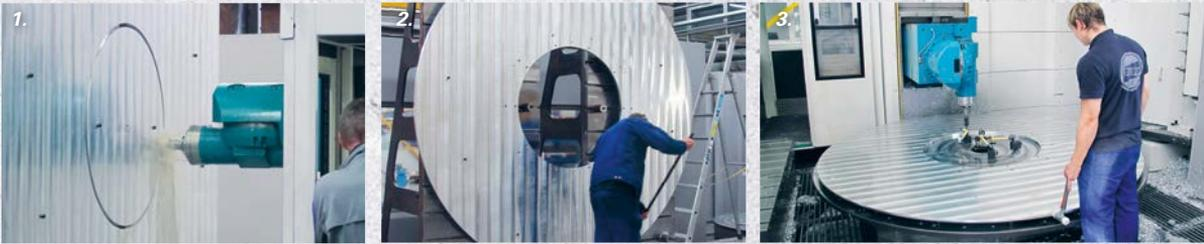
**1./2. The first operation creates the round plate from a square cast aluminium block. The flat surfaces are then milled in multiple steps – to establish the necessary thickness. 3. In the first milling step, the rotary table surface is produced. This is then followed by the remaining areas. The plate itself is continually realigned between the various steps to ensure a precise finish.**
