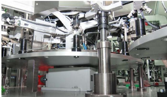
**Rotary table 1, a user-programmable NC320 supplied by WEISS, is at the heart of the system: it brings the seal and springs together and forwards the components to the other tables.**
