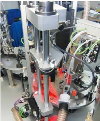
**Both spring rings are placed into the seal during two circuits on table 2. The user-programmability of the NC 150 permits the required intermediate processing stage.**
