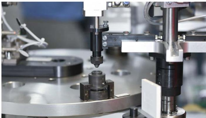
***The assembly of sealing rings for injection pumps requires maximum precision. This is ensured by rotary indexing tables and coordinated rotating plates supplied by WEISS.***
